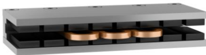
Abb. 7 Structure of a linear motor: Three current-carrying magnetic coils move in a magnetic track or vice versa
