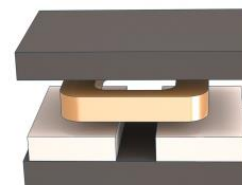
Abb. 2 Voice coil motor with a flat design
